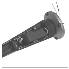
**3.** Remove half fixture. Remove transformer and replace with new transformer. Reassemble fixture in opposite order.
