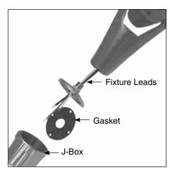
3. Thread fixture leads through coupling and install fixture. Attach fixture leads to circuit leads observing polarity, i.e., green-to-ground, white-to-common, and black-to-voltage.
